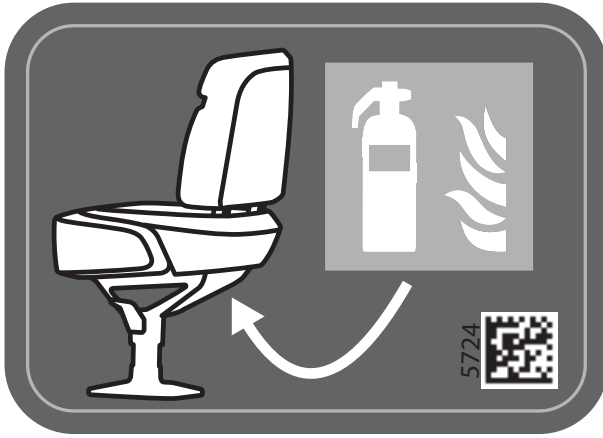
FIRE EXTINGUISHER POSITION LABEL
