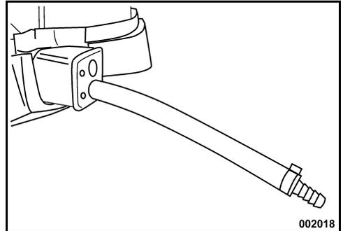
1. Flexible et raccord de carburant – 9 mm (3/8 po)
