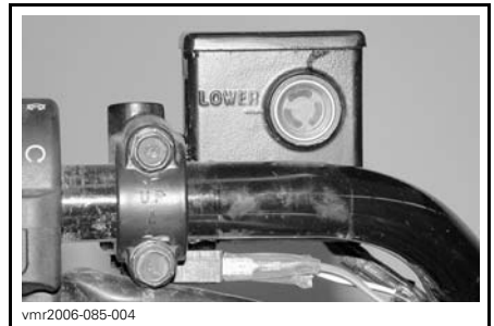
TYPICAL — LH REAR BRAKE FLUID RESERVOIR
