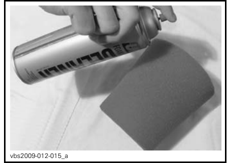
TYPICAL - SPRAY FOAM ELEMENT INSIDE AND OUT
