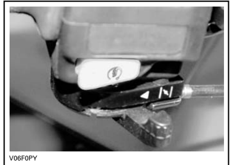
CHOKE LEVER IN THE OFF POSITION
