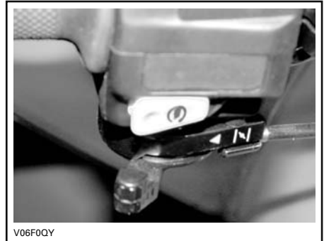
CHOKE LEVER IN THE FULL CHOKE POSITION
