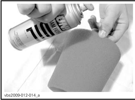
TYPICAL - OIL THE FOAM FILTER ELEMENT
