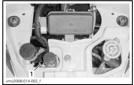
TYPICAL 1. Coolant reservoir
