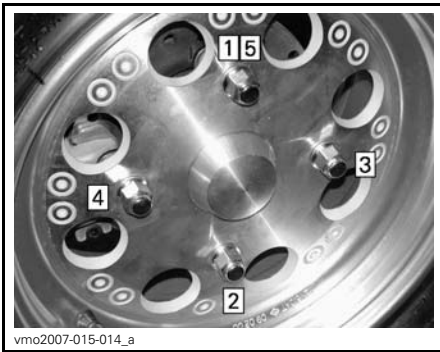
TIGHTENING SEQUENCE
