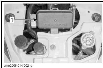
1. Front fuses box
