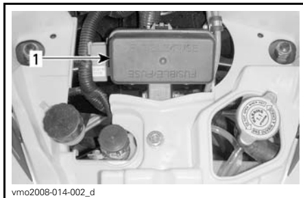
1. Front fuses box
