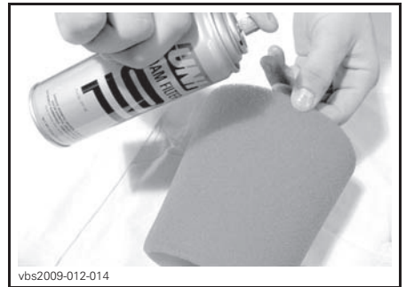
TYPICAL - OIL THE FOAM FILTER ELEMENT
