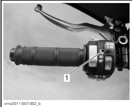
1. Emergency engine stop switch
