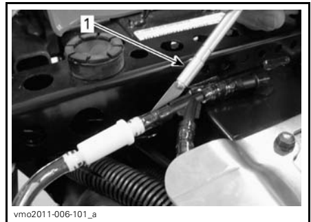
TYPICAL - CAREFULLY CUT HOSE
