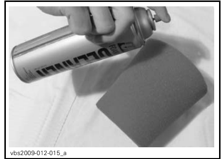
TYPICAL - SPRAY THE FOAM ELEMENT
