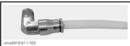
HOSE PROPERLY INSERTED INTO FITTING
