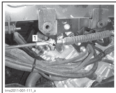
LH SIDE — FRONT CYLINDER 1. Spark plug
