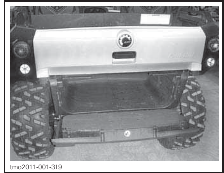
TYPICAL - LOWER SECTION WITH LOWER TAILGATE
