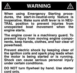
If the electric starter fails or the battery's voltage is too low to power the starter, use the cord from the tool kit and these instructions to start your engine manually.
