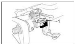
1. Tilt lock lever - RELEASE position
