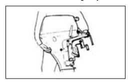
The resulting position of the anti-ventilation plate must be 0 to 1 in. (0 to 25 mm) below the boat's bottom.
