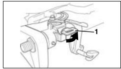
Tilt lock lever – RELEASE position
