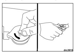
Connect the clip to the emergency stop/key switch. Snap the lanyard to a **secure** place on the operator's clothing or life vest — not where it might tear away instead of activating the stop switch.
