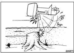
The engine's shock absorption system does not work while operating in reverse. If you back into an object, either in the water or while trailering, your boat and engine can be seriously damaged.
