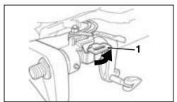
1. Tilt lock lever - RELEASE position
