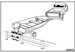
If you hit any object, stop immediately and examine the engine for loosening of attaching hardware and clamp screws, if equipped. Inspect for damage to swivel and stern brackets, steering components, and components in the area of impact. Also, examine the boat for structural damage. Tighten any loosened hardware. If the collision occurred in the water, proceed slowly to harbor. Before boating again, have your Dealer thoroughly inspect all components.
