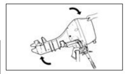
Slowly, lower motor until shallow-water drive bracket rests against angle adjusting rod.
