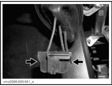
PUSH ON LOCKING TAB TO UNLOCK CONNECTOR
