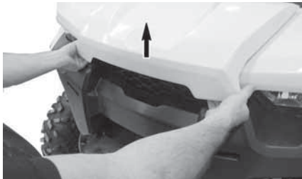
LIFTING FRONT SERVICE COVER EDGE.
