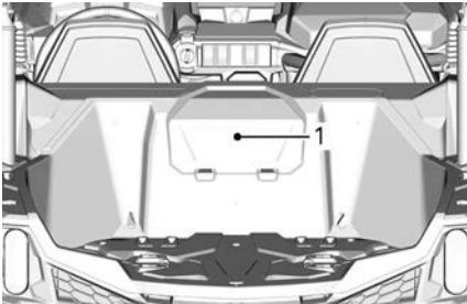
1. Coolant tank access cover
