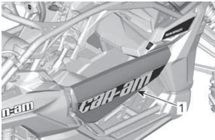
1. Door closed and locked in place
