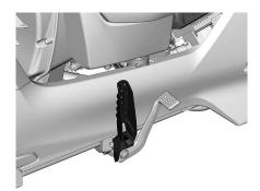
Slide the footpeg and the brake pedal forward or rearward to the desired position.
