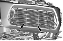
4. Roll up the end of the front fascia extensions to release the rear retaining tabs.
