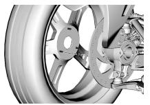
Install the conical washer and the center lock wheel nut.
