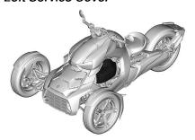
The left service cover must be removed to servicing the engine air filter.
