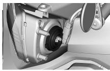
Turn the bulb stopper counterclockwise to unlock it.
