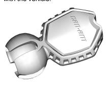
Each key contains an electronic circuit including a specifically pre- programmed chip that is read via radio frequency by the immobilizer system to allow starting the engine.
