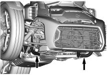
USE THESE TUBES TO LIFT OR SUP-PORT THE FRONT OF THE VEHICLE
