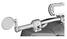
It turns off automatically after a normal turn, but you may have to turn it off manually after a shallow turn or lane change.
