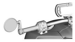
Press the button to activate the horn.
