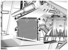
4. Remove the air filter from its housing.
