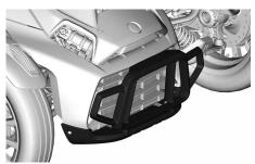
Remove screws located underneath the front fascia.
