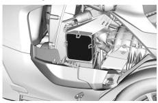
Remove the screw retaining the bottom of the CVT air filter housing.
