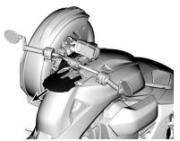
Unscrew slowly the fuel reservoir cap counterclockwise to remove it.
