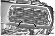
Tighten screws located underneath the front fascia to specification.
