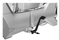
4. Lower the footpeg and validate that the driver is able to apply the full stroke of the brake pedal.
