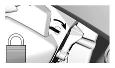
To unlock the park position lever, turn key counterclockwise.
