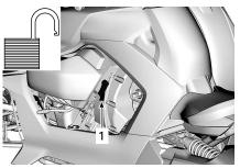
1. PARK lever in unlock position (disengaged)
