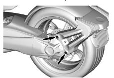
7. Remove the center lock wheel nut and the conical washer.
