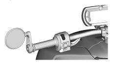
This switch is used to select either the headlights low or high beams
