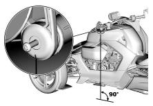
5. Hold the support and tighten the screw.
