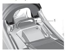
1. Retaining bar Installing the Seat
