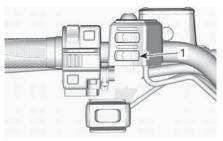
1. Heated throttle lever switch
