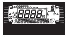
Display the vehicle speed in km/h or MPH.
