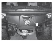
1. Rear storage compartment latch Closing the Rear Storage Compartment
