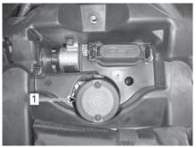
1. Rear brake fluid reservoir **Adding Brake Fluid**
