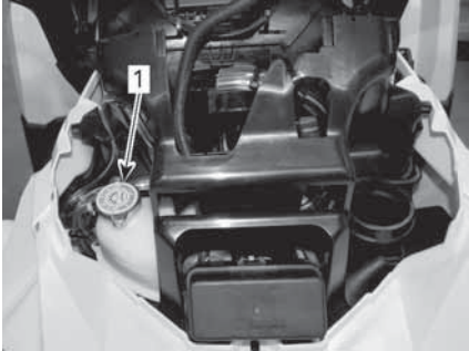
1. Engine coolant reservoir
