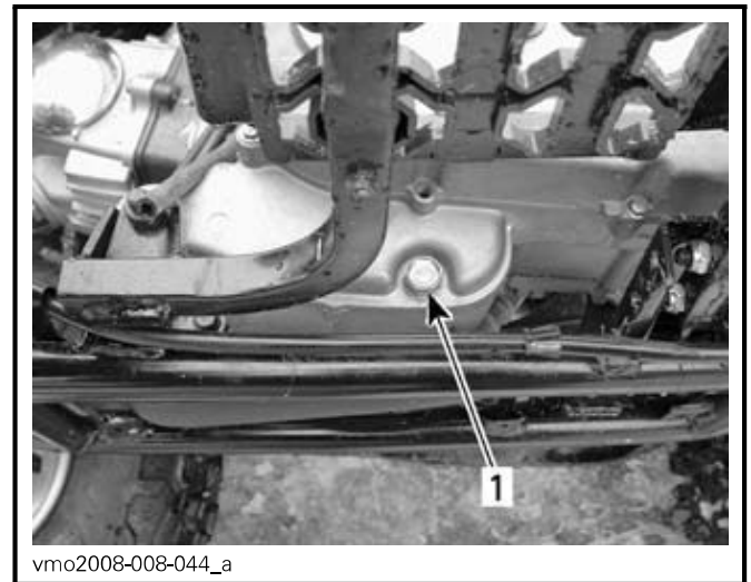
LH SIDE OF ENGINE 1. Drain plug
