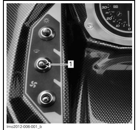
1. Bilge pump switch
