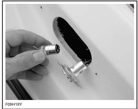
TYPICAL — PUSH IN, TWIST AND REMOVE BULB
