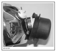
Unlock the bulb socket.
