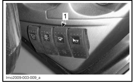
1. Bilge pump switch
