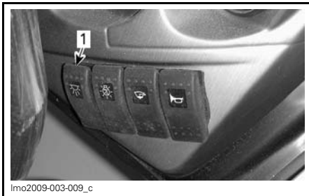
1. Deck light switch
