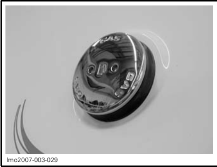
TYPICAL - FUEL TANK CAP
