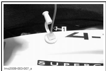
1. Can needle into lubrication fitting
