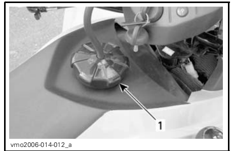
TYPICAL 1. Fuel tank cap
