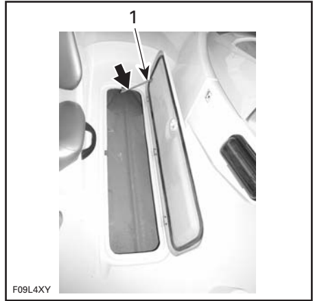
TYPICAL 1. Gently push here to release the spring
