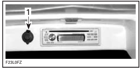
LOCATED IN THE GLOVEBOX — 180 CHALLENGER 1. 12-volt jack
