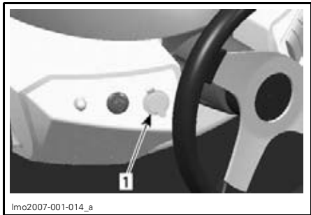
TYPICAL — LOCATED ON DRIVER'S CONSOLE — 150 SPEEDSTER 1. 12-volt jack
