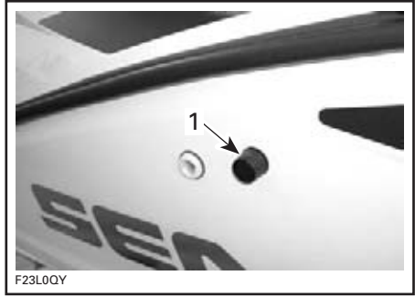
TYPICAL — 180 CHALLENGER 1. Fuel tank vent
