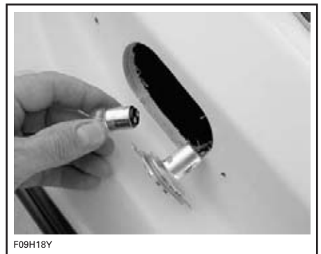
TYPICAL — PUSH IN, TWIST AND REMOVE BULB
