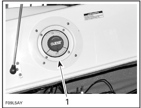
TYPICAL — SPORTSTER 4-TEC — MAIN BATTERY CUT-OFF SWITCH
