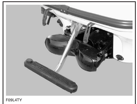
TYPICAL — LADDER LOWERED — SPORTSTER 4-TEC
