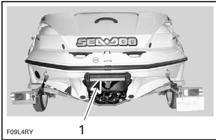
TYPICAL 1. Retractable ladder
