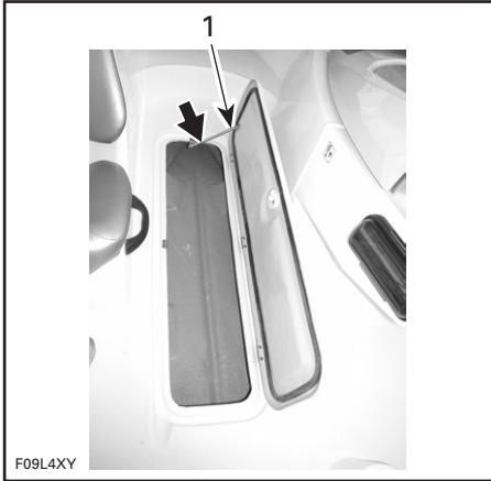
TYPICAL 1. Gently push here to release the spring
