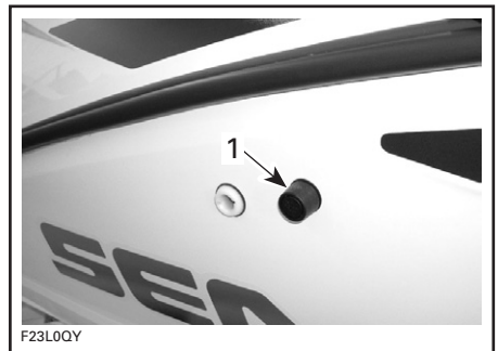
TYPICAL — CHALLENGER 180 1. Fuel tank vent
