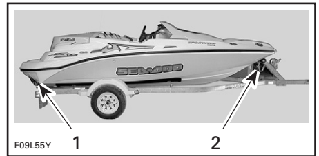
TYPICAL 1. Stern eyelet 2. Bow eyelet
