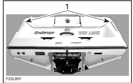
TYPICAL 1. Ventilation ducts
