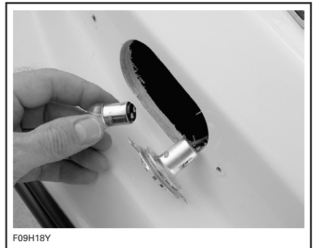
TYPICAL — PUSH IN, TWIST AND REMOVE BULB
