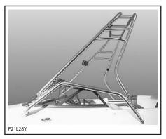
**CAUTION:** Always tow the vehicle with the towing tower fastened in the upright position to avoid damage to the boat and towing vehicle while in transport. Tower must be secured and in the upright position to avoid damage to the boat. Periodically check that bolts are in place and tight. Check clearance height around docks, shore, overhanging objects, bridges and power lines. The tower must not be used as a tie-down or tie-off point.
