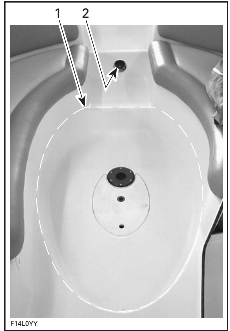
1. Foot well surface 2. Wash down valve
