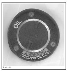
To add injection oil in the reservoir, unscrew the cap counterclockwise.
