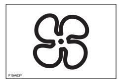
A 2-position push type switch. When ON, it ventilates the engine compartment.
