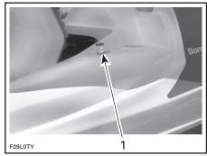
**TYPICAL — SPEEDSTER SHOWN** 1. Flushing connector with its cap
