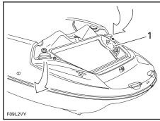
**TYPICAL — AIR FLOW** Bilge air blower inside engine compartment
