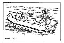
Always activate air blower switch four minutes before starting the engine.
