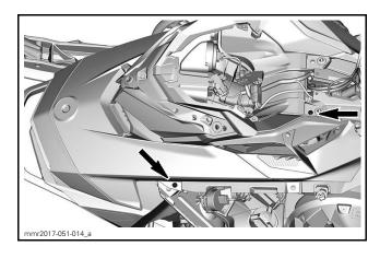
9. Free the rear end hooks of the upper body module from the slots in the console.
