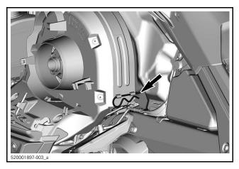
Lift rear portion of guard then release from front tab.
