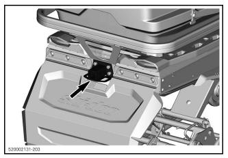
Use the hitch in conjunction with a tow bar to tow an accessory.
