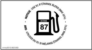
LOCATED ON FUEL CAP - ON 600 ACE AND 900 ACE ENGINE (IN COUNTRIES USING PUMP POSTED AKI (RON+MON)/2 OCTANE RATINGS)
