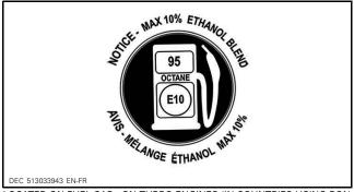
LOCATED ON FUEL CAP - ON TURBO ENGINES (IN COUNTRIES USING RON OCTANE RATINGS)
