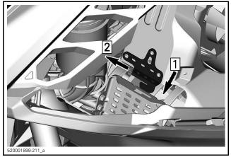
Step 1: Lower belt guard Step 2: Slide belt guard
