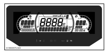
Display the vehicle speed in Km/h (or MPH) or the RPMs. Refer to SETTINGS
