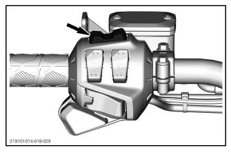
Press the MENU (M) button to cycle through suspension settings.
