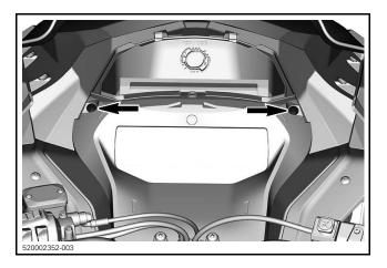
3. Lift the front of the gauge support, then slide it forward to remove it
