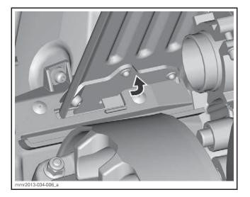
Position the rear portion of the belt guard over the retainer and secure it using the retaining pin.
