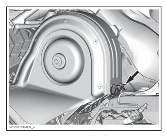
Lift rear portion of guard then release from front tab.
