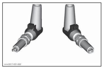
6. Remove spark plug cables as shown.
