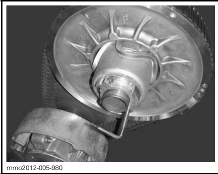
PULLEY EXPANDER INSTALLED ON ADJUSTER HUB
