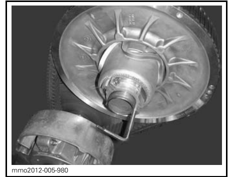
PULLEY EXPANDER INSTALLED ON ADJUSTER HUB
