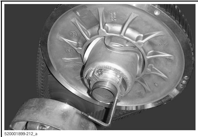
TYPICAL - PULLEY EXPANDER INSTALLED ON ADJUSTER HUB
