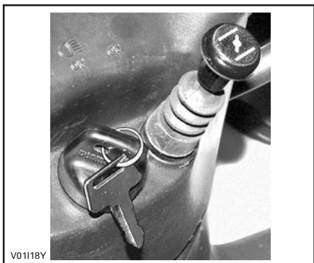
CHOKE LEVER IN THE FULL CHOKE POSITION
