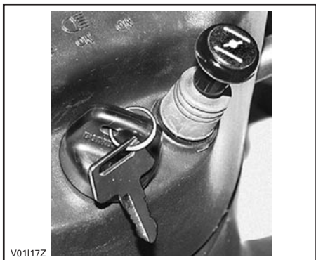
CHOKE KNOB LEVER IN THE OFF POSITION
