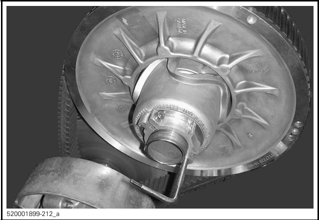
TYPICAL - PULLEY EXPANDER INSTALLED ON ADJUSTER HUB
