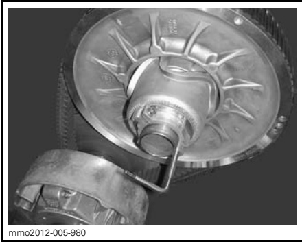
PULLEY EXPANDER INSTALLED ON ADJUSTER HUB
