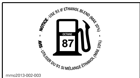
LOCATED ON FUEL CAP - ON 550F, 600 ACE AND 900 ACE ENGINES (IN COUNTRIES USING PUMP POSTED AKI (RON+MON)/2 OCTANE RATINGS)
