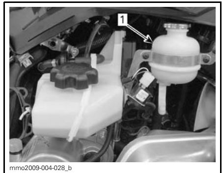
TYPICAL 1. Coolant tank
