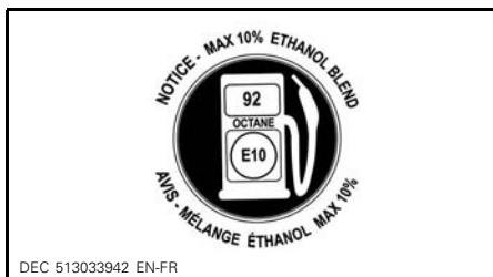
LOCATED ON FUEL CAP - ON 550F, 600 ACE AND 900 ACE ENGINES (IN COUNTRIES USING RON OCTANE RATINGS)
