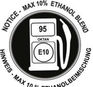
A circular fuel tank cap label. In the center is a fuel pump icon with the number '95' and the word 'OKTAN' above it. Below the pump icon is 'E10'. The text 'NOTICE - MAX 10% ETHANOL BLEND' is written around the top inner edge. The text 'HINWEIS - MAX 10 % ETHANOLBEIMISCHUNG' is written around the bottom inner edge.
