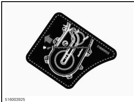
CHAIN CASE OIL VERIFICATION- EUROPEAN MODELS
