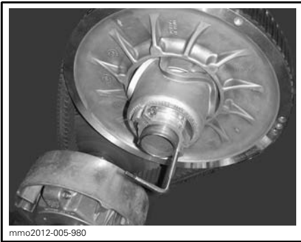
PULLEY EXPANDER INSTALLED ON ADJUSTER HUB
