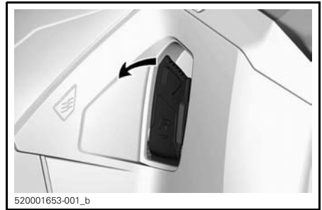
PULL TO ENGAGE REVERSE GEAR
