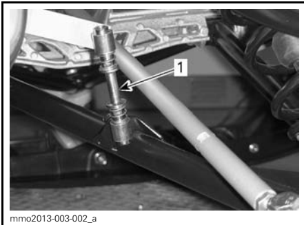
TYPICAL 1. Quick disconnect
