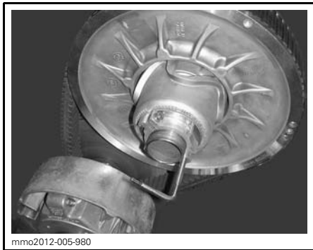
PULLEY EXPANDER INSTALLED ON ADJUSTER HUB
