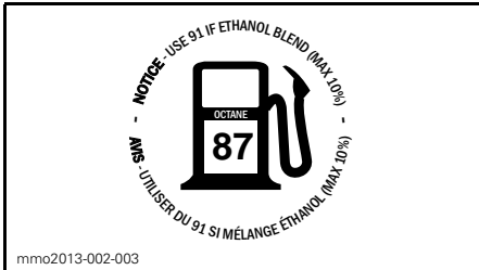
LOCATED ON FUEL CAP - ON 550F AND 600 ACE ENGINES (IN COUNTRIES USING PUMP POSTED AKI (RON+MON)/2 OCTANE RATINGS)
