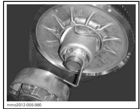
PULLEY EXPANDER INSTALLED ON ADJUSTER HUB
