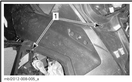
LH SIDE SHOWN 1. Retaining screws
