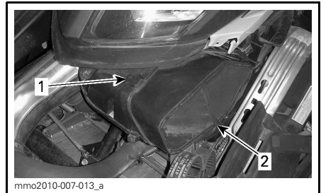
1. Retaining clip 2. Air filter
