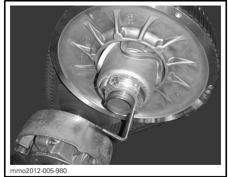
mmo2012-005-980 PULLEY EXPANDER INSTALLED ON ADJUSTER HUB
