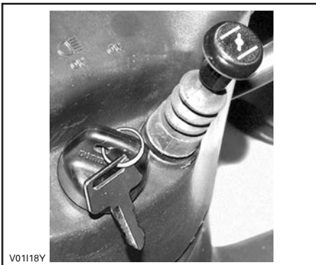
CHOKE LEVER IN THE FULL CHOKE POSITION
