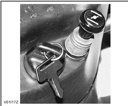
CHOKE KNOB LEVER IN THE OFF POSITION
