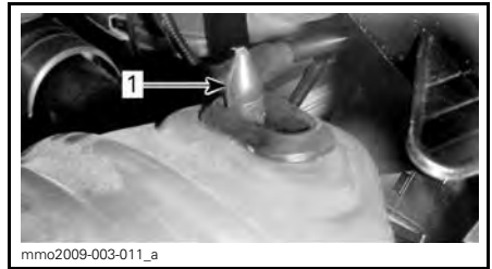
TYPICAL 1. Retaining rod
