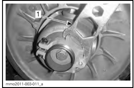
1. Suspension adjustment tool
