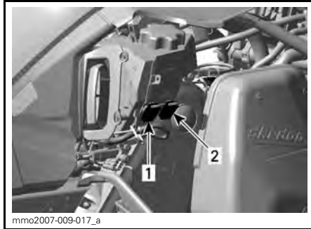
RH SIDE OF ENGINE COMPARTMENT 1. 15 A headlight fuse (RED/ORANGE wire) 2. 20 A accessories fuse (RED/YELLOW wire)
