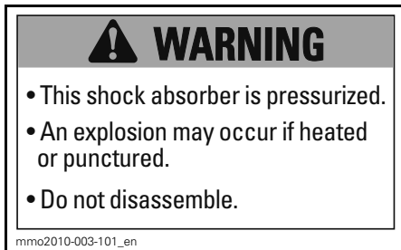
LABEL 14 - ON SHOCK GAS CHARGED ABSORBERS
