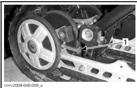
1. RH adjustment screw
