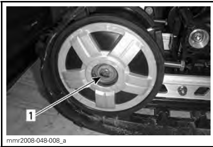
1. RH rear idler wheel retaining screw
