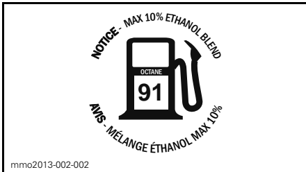
LOCATED ON FUEL CAP - COUNTRIES USING PUMP POSTED AKI (RON+MON)/2 OCTANE RATINGS
