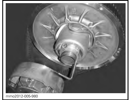
PULLEY EXPANDER INSTALLED ON ADJUSTER HUB
